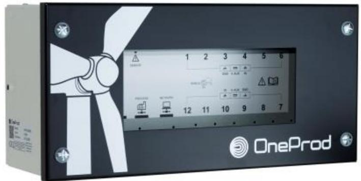
More than 60% of ONEPROD's systems are installed in wind turbines: **KITE** has been designed to offer optimized monitoring of wind turbines. Its 12 acquisition channels make it possible to monitor the drivetrain, structure and nacelle. Faults are identified with great accuracy months before maintenance work is required, including in relation to the gearbox.
